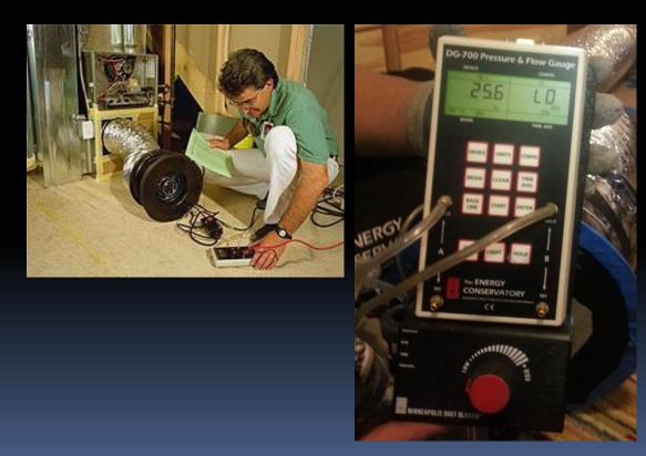
Conditioned Floor Area divided by 100 x Code Max Leakage CFM
