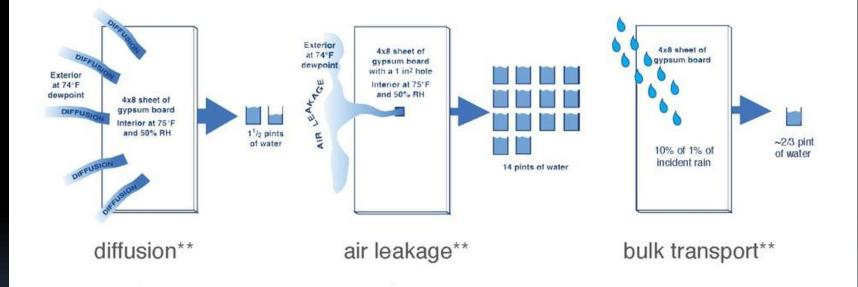
"Diffusion & air leakage graphic courtesy of Lstiburek, "Builder's Guide to Hot Humid Climates" (2006); bulk transport graphic
