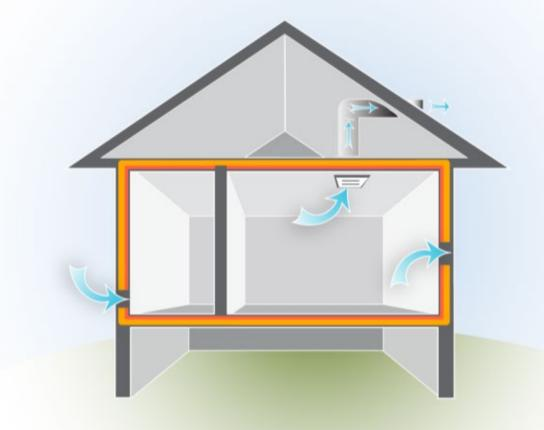
Infiltration = Air leaking in
